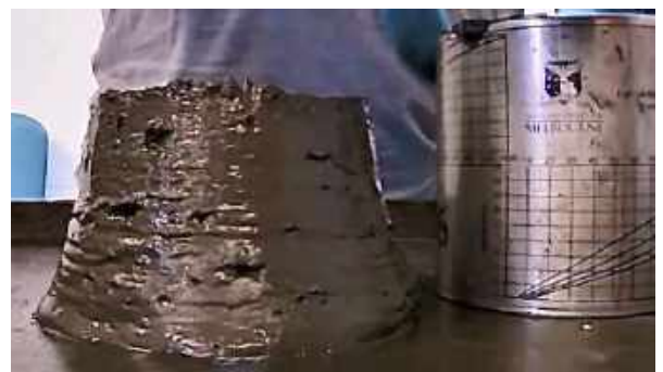
Slump test, solid content > 75%
