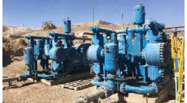
ABEL HMQ for the transfer of copper tailings on 7 km
