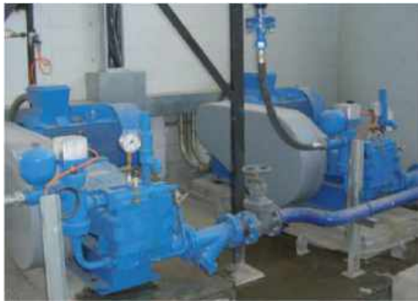
ABEL HP-K-25 for filter cloth cleaning of chamber filter presses
